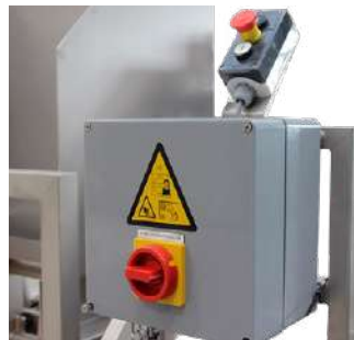
Operator/control panel with emergency stop.
