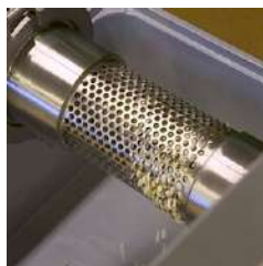
Cheese extrusion filter comes with varied filter sizes, typically \varnothing 2.8 , \varnothing 5 and \varnothing 14 mm.
