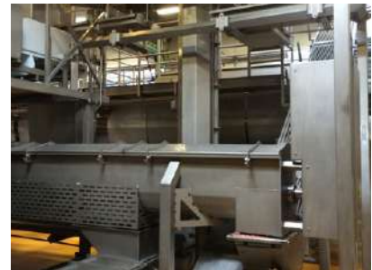
scansteel foodtech ® Whole Pallet Crusher, WPC 2000-Single, shown in application where existing footprint is sparse and where the pre-broken frozen blocks must be elevated to approx. 5000 mm.
