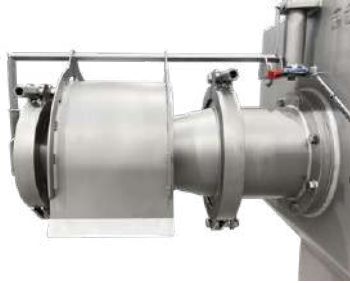
Extruder filter shown without safety cover.
