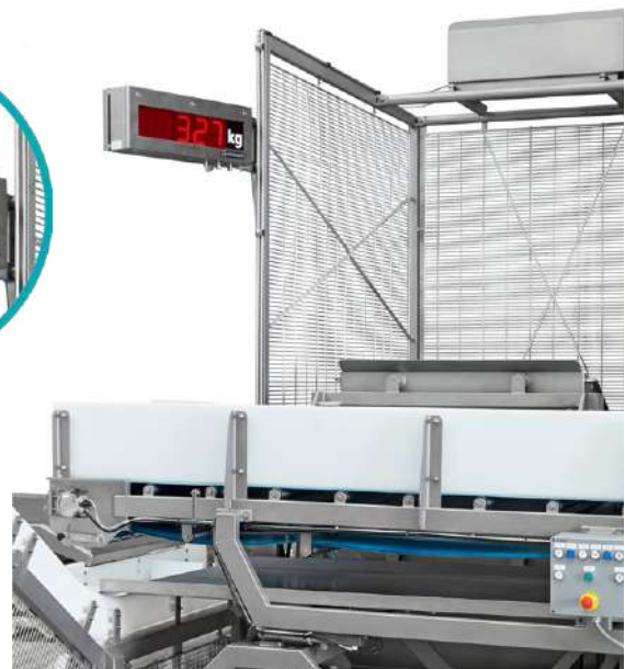
Details showing drip trays and weighing/load cells.
