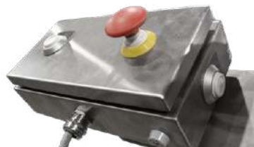
Close up view of operator panel with two hand JOG function for cleaning and inspection.
