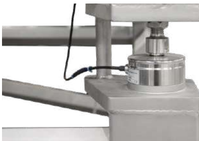
Close up view of load cells.
