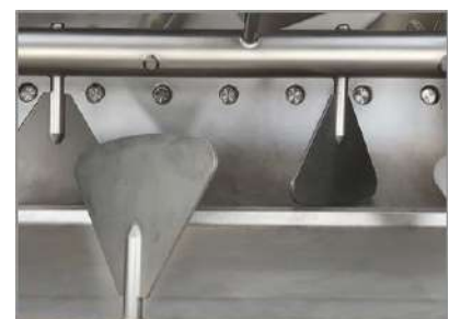
Paddle mixing wings, special application.
