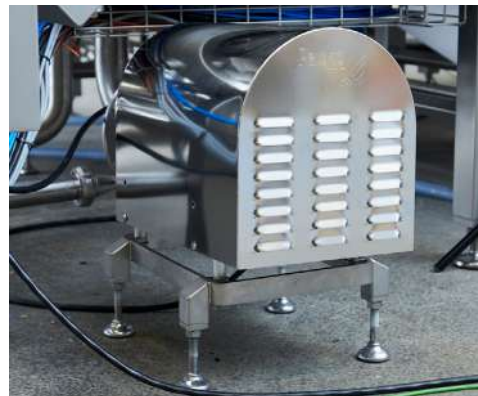
Pumps are positioned/mounted on their own frame for easy access at inspection/maintenance, etc. In addition, the pump of the scanGravy mixing unit can be equipped with its own knife system for eliminating lumps in “challenging to produce” gravies.
