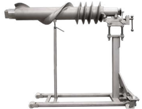
Cleaning trolley for worm/auger shown with safety shaft mounted for cleaning, inspection, and transport.
