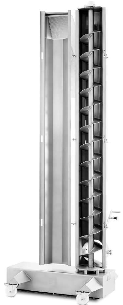
scansteel foodtech® standard scanGiraff, showing vertical screw.
