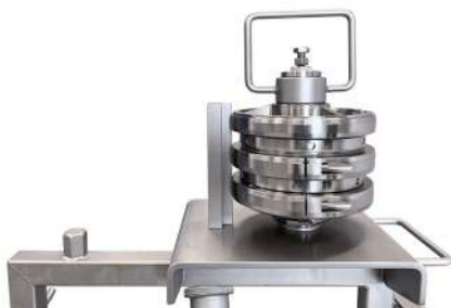
Knife cassette of scanEmul 175 - Hopper fed shown assembled.
