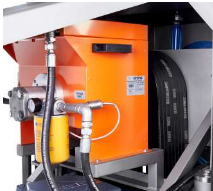
Built-in oil coolers for gear box dramatically increase life time of the gear box.
