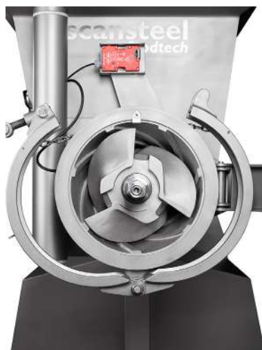
Front end of SuperGrind 400/260 shown disassembled, with worm/auger in place, ready for mounting of 3-bladed cut-knife. Cut-knife recessed into the worm/auger.
