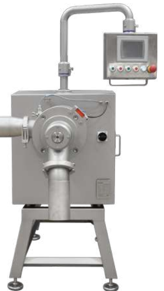
Superpump SP 250 shown below feeding a scanDebone 150.
