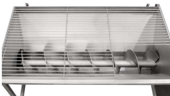
Infeed hopper shown with safety guard/grill in running position.
