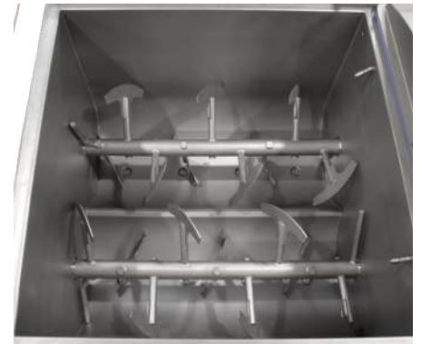
Inside view of scansteel foodtech® Twin Shaft Mixer, TSM(V)
