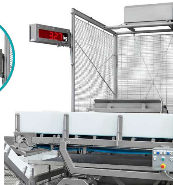
Details showing drip trays and weighing/load cells.
