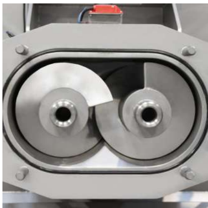
Close up view of twin screws, front view. Another use is simply read.
