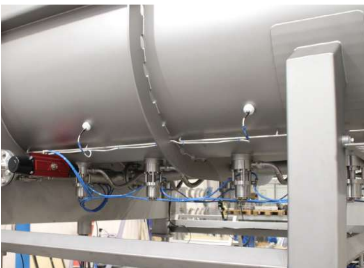
Close up of scansteel foodtech® Bottom steam injection system shown on Twin Shaft Mixer, TSM(V)
