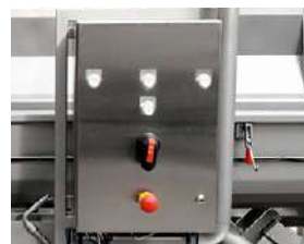
Standard screw conveyor electrical/operator panel.
