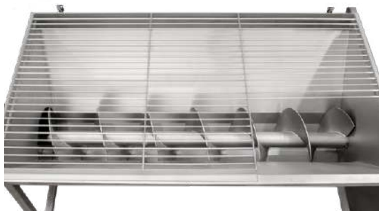
Infeed hopper shown with safety guard/grill in running position.
