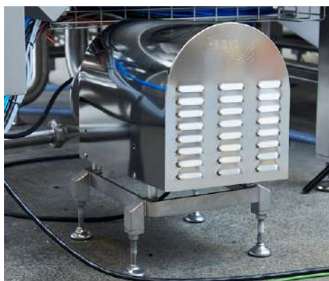
Pumps are positioned/mounted on their own frame for easy access at inspection/maintenance, etc. In addition, the pump of the scanGravy mixing unit can be equipped with its own knife system for eliminating lumps in "challenging to produce" gravies.
