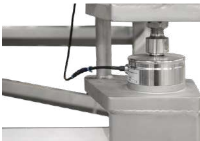
Close up view of load cells.
