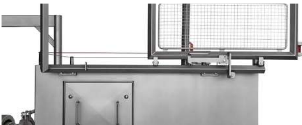
Top picture: Safety guard for platform shown in running position. Bottom picture: Safety guard for platform shown in open/cleaning/inspection position.
