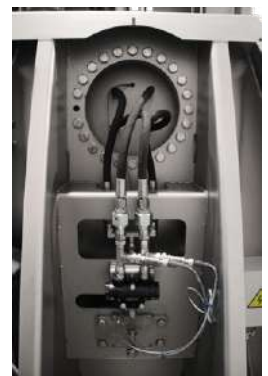
Pallet inverter seen from behind without cover, view of hydraulic unit and turning device.
