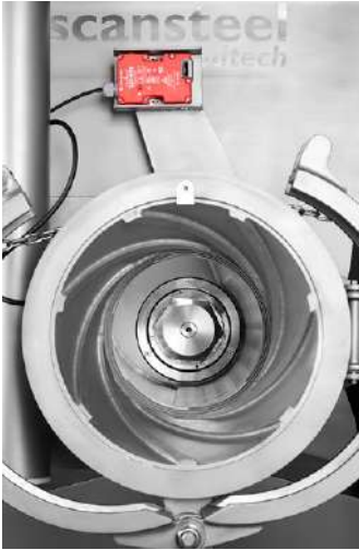
Cabinet without worm/auger showing the flights of the lining.
