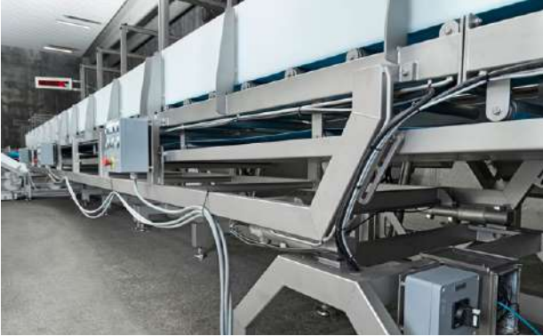
Belt conveyors with a range of standardized side rails and drip pans to avoid moisture and liquids on the floor.
