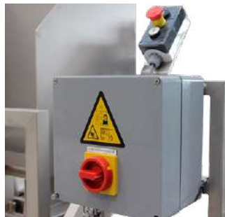
Operator/control panel with emergency stop.
